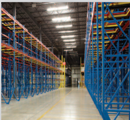
Lowest rail slope means less push back force required
