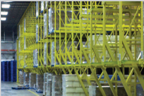
Rails are a single welded unit with 4" notched arms
