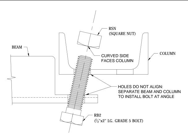
C3 & C4 BEAMS: (1) BOLT EA. END (U.N.O.) C5 & C6 BEAMS: (2) BOLTS EA. END RECOMMENDED TORQUE RANGE IS 45 TO 80 FT.LBS.
